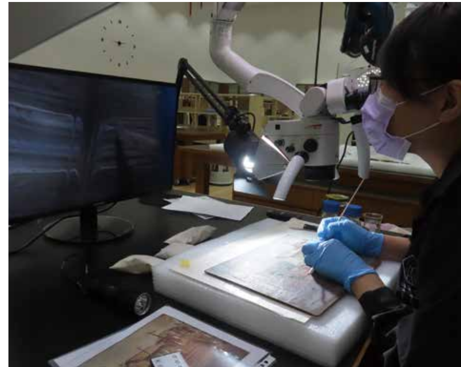
Using a surgical microscope to carefully remove termite excrements and clean the art work.
